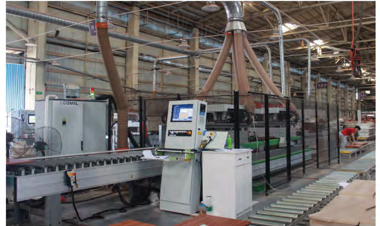
Germany HOMAG electronic automatic four-side edge banding machine
